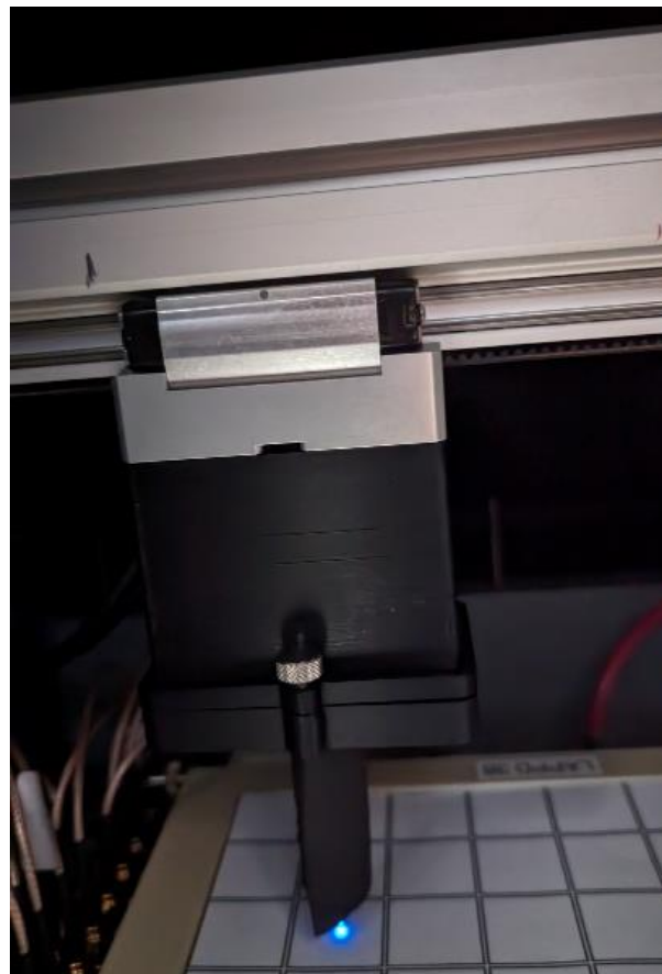
Photo of optical fiber installed in LED box and covered with black foam, left. Powered LED over the LAPPD window, right
