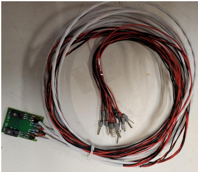
HTSB with humidity and temperature sensors and cables
